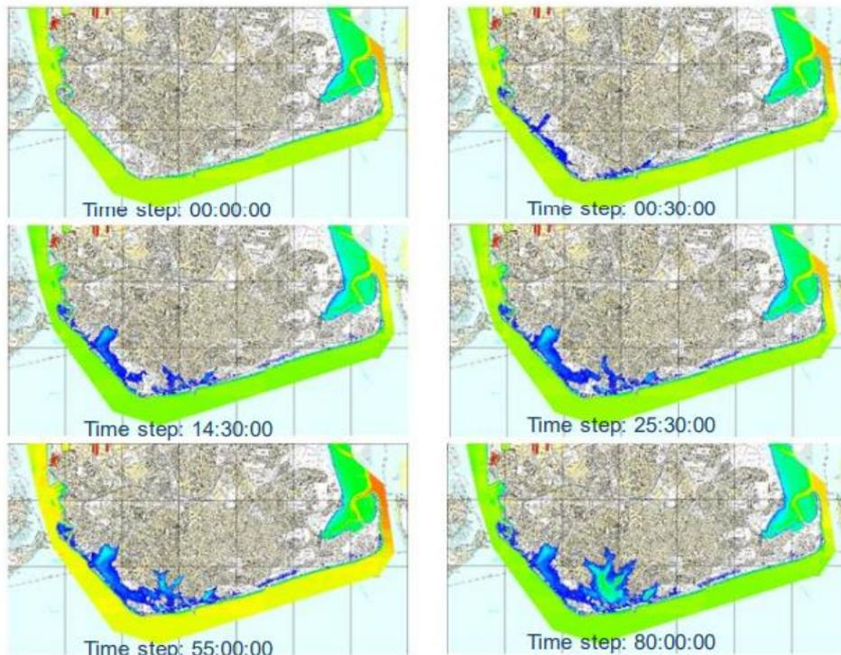
These models have been carried out for a range of scenarios to simulate different levels of extreme events, to see the spread of the flood, and the depth of the flood within the area.
